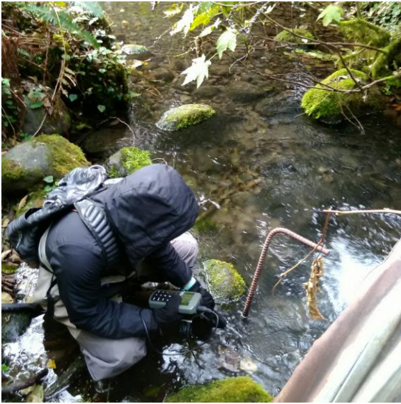
Figure 5. Collecting dissolved oxygen data at WCT01.
