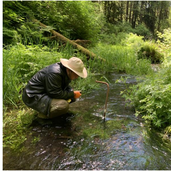
Figure 6. Downloading temperature data from the in-stream logger at WCT02.
