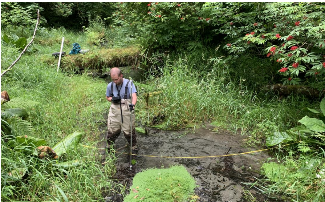
Figure 11. Measuring flow velocity at WCT03.
