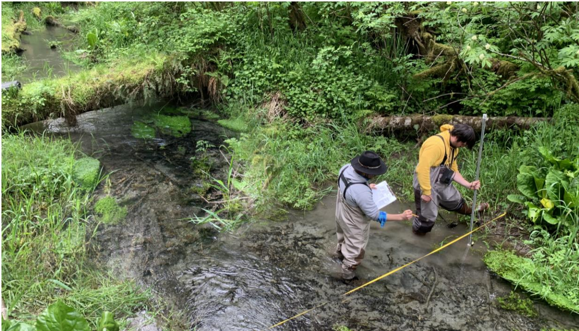
Figure 3. Measuring stream velocity at WCT03.
