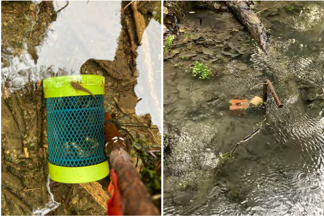
Figure 3a. (left) Original housing for the HOBO Pendant™ temperature logger consisted of a crab bait cage attached to rebar by several exterior use zip-ties. Figure 3b. (right) Updated housing consists of a 2” PVC pipe covering for the temperature logger and a half brick to weight the system. The system is attached to rebar via tar-coated parachute cord. These updates were implemented on October 7, 2020.
