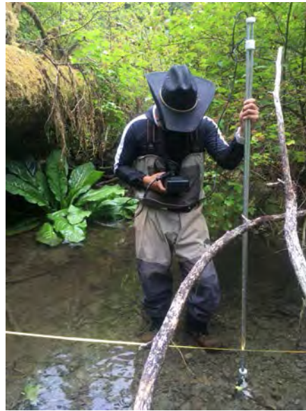
Figure 4. Field technician Miguel Rodriguez sampling flow in Irely Creek using a Swiffer flow meter (Model 3000) on July 3, 2020.
